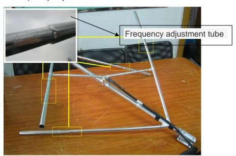
Frequency adjustment tube, Make A1, A2, B1, B2 oscillators frequency be consistent with the transmitter frequency
